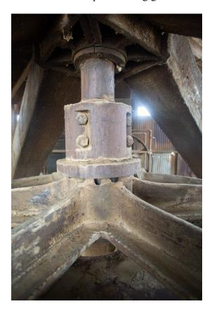
**Photo 20** Jack Plant machinery showing the ring gear at the bottom and its surrounding oil pan, the vertical shaft, eccentric gears and wood timber framework. The camera is facing east.
