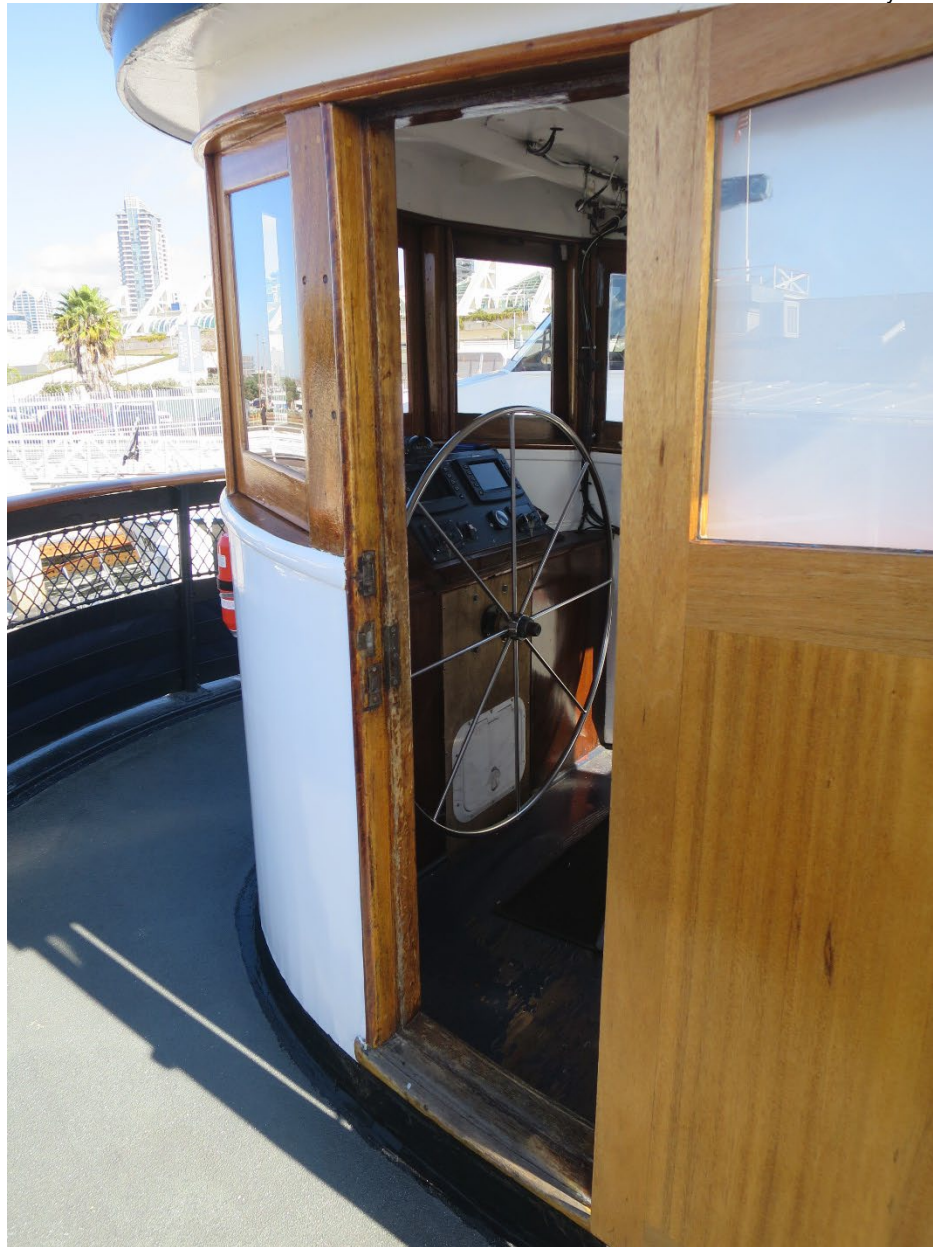
Photo 16. Silvergate , pilothouse, starboard view showing helm and navigational console
